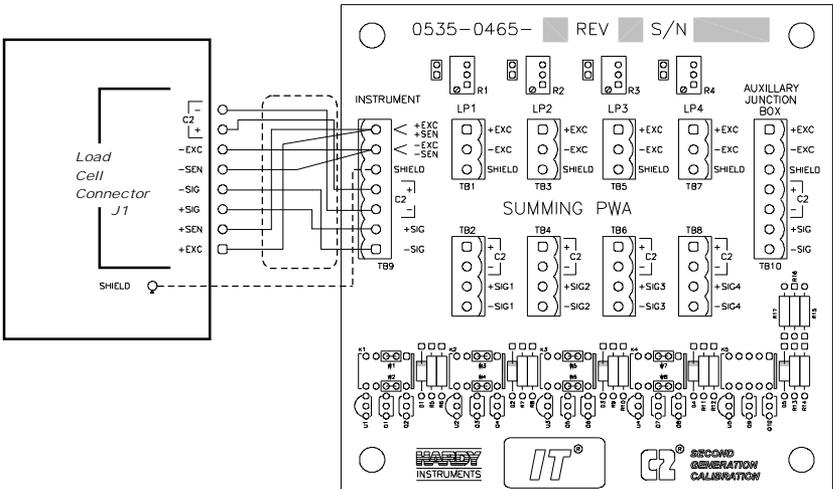
**FIG. 3-14 HARDY HI 215IT JUNCTION BOX WIRING DIAGRAM**
