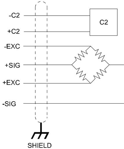
FIG. 3-7 HARDY LOAD SENSOR/C2 WIRING
