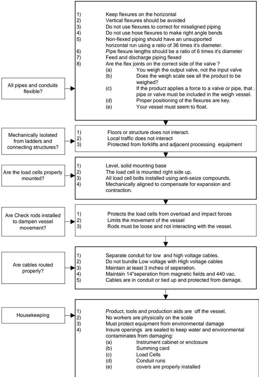
**FIG. 7-3 MECHANICAL INSPECTION**
