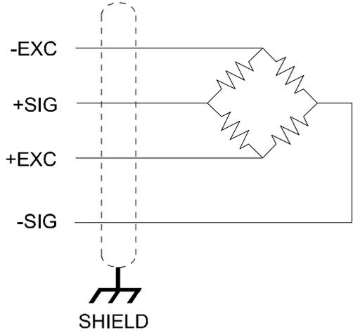
FIG. 3-6 INDUSTRY STANDARD LOAD CELLS
