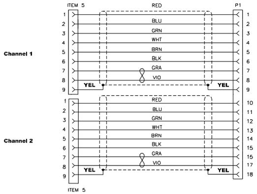
**FIG. 3-13 RTA CABLE SCHEMATIC - HI 1756-2WS DUAL CHANNEL**
