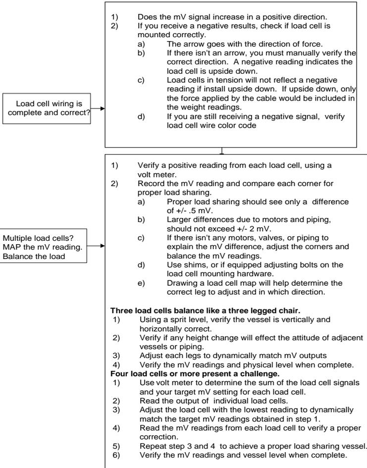
**FIG. 7-4 LOAD SHARING AND LOAD SENSOR CHECKOUT**
