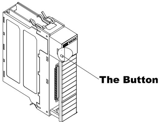
**FIG. 5-4 “THE BUTTON” C2 CALIBRATION - HI 1756-2WS**
