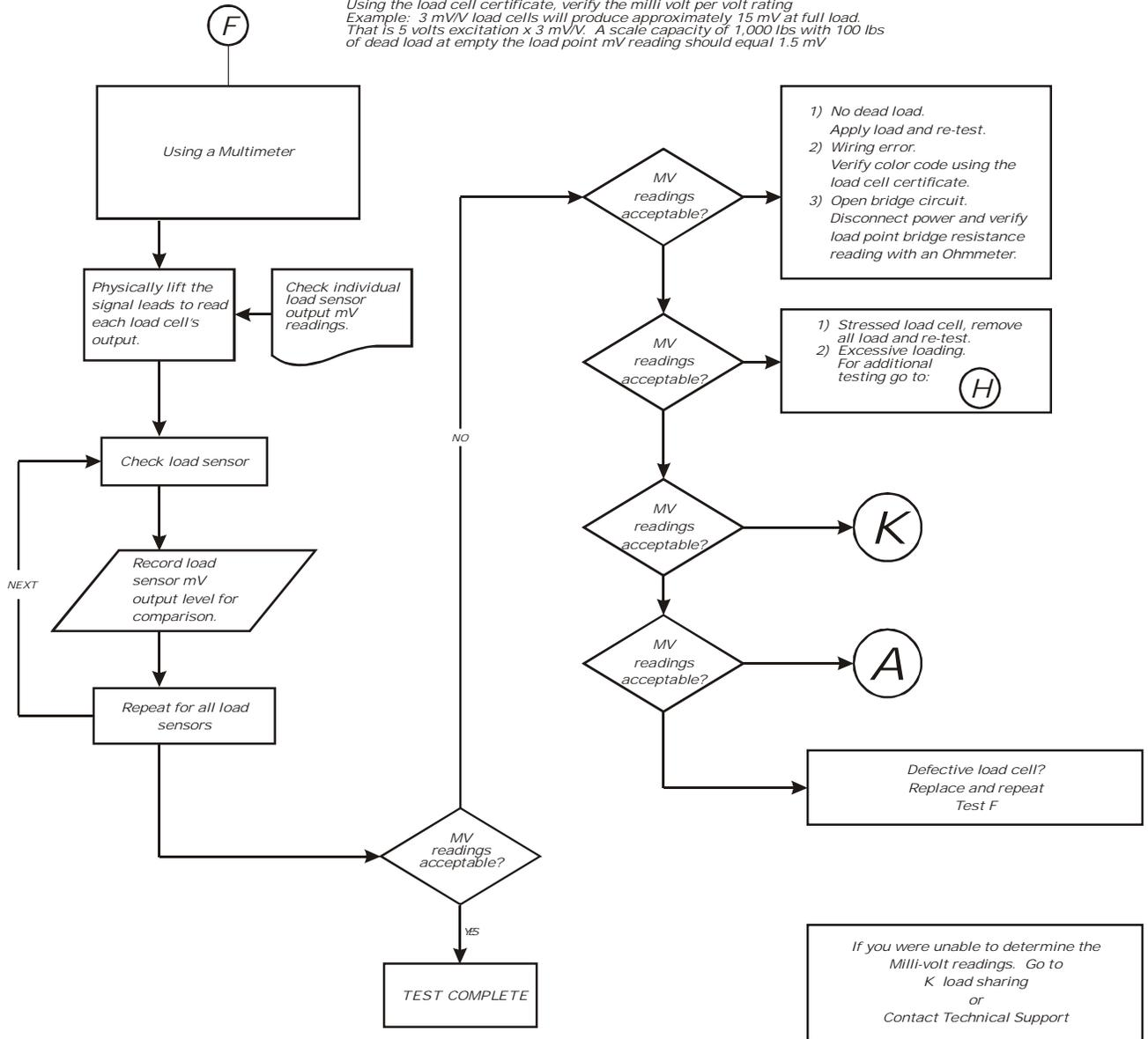
**F(a) - Verify Individual Load Cell Readings Using Diagnostics**
