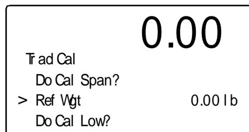
**FIG. 5-7 CALIBRATION ENTERING REFERENCE WEIGHT**
