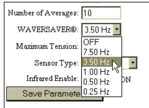
**FIG. 4-60 INSTRUMENT SETUP PAGE/SELECTING WAVERSAVER SETTING**
