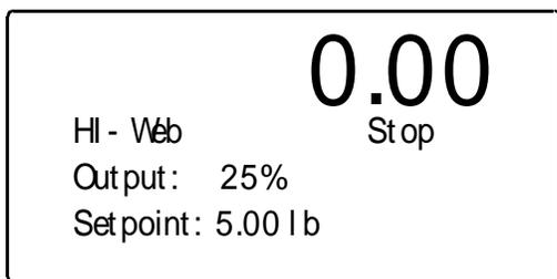
**FIG. 4-7 FRONT PANEL/OPERATING MODE DISPLAY/STOP**
