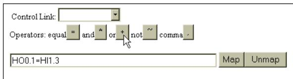
**FIG. 6-24 HIGH TENSION ALARM (HI1.3) ADDED TO THE MAP FIELD**
