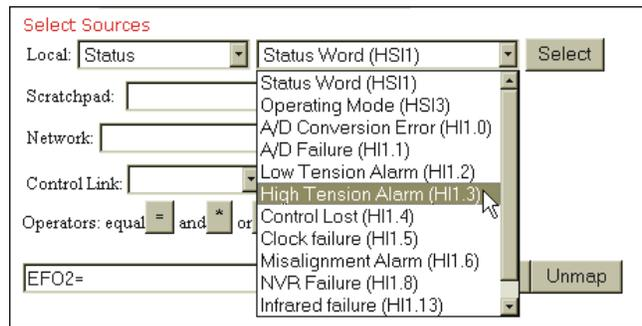
**FIG. 6-8 STATUS SOURCE PULL DOWN MENU/SELECTING HIGH TENSION ALARM (HI1.3)**
