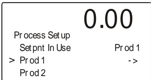
FIG. 4-31 PROCESS SETUP MENU/SETTING PROD 1 PARAMETERS
