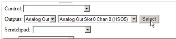
**FIG. 4-83 SELECTING ANALOG OUT SLOT 0 (HSO5)**
