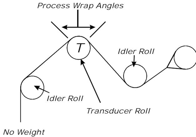
FIG. 5-8 CALIBRATION SETUP WITH NO WEIGHT
