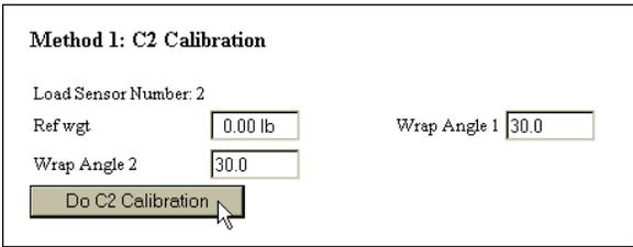
**FIG. 5-33 METHOD 1: C2 CALIBRATION**
