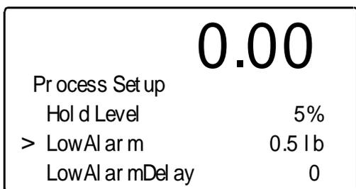
**FIG. 4-44 INSTRUMENT SETUP MENU/SETTING LOW ALARM**
