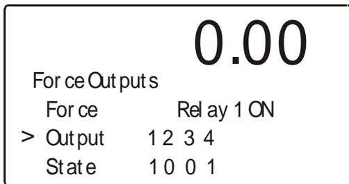
**FIG. 7-9 FORCE OUTPUTS MENU/READING OUTPUT 1234**
