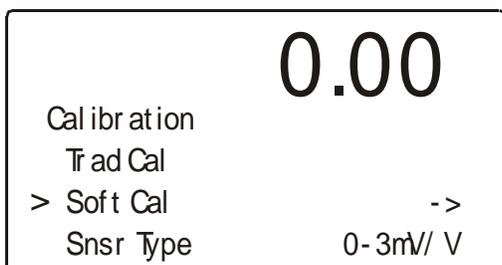
**FIG. 5-13 CALIBRATION MENU/SELECTING SOFT CALIBRATION**
