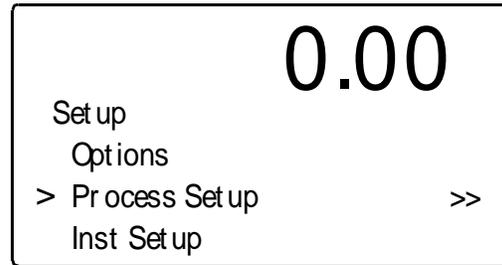
**FIG. 4-28 SETUP MENU/SELECTING PROCESS SETUP**
