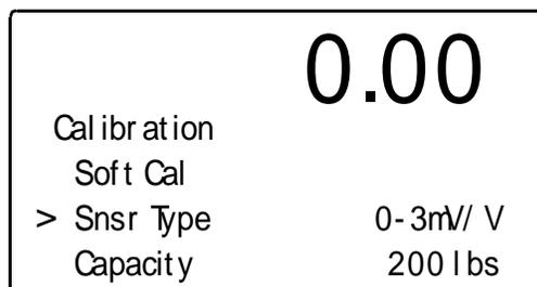
**FIG. 5-23 CALIBRATION/SELECTING SENSOR TYPE**
