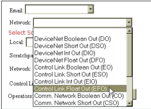
**FIG. 6-4 SELECTING DESTINATION/NETWORK/CONTROL LINK FLOAT OUT (EFO)**
