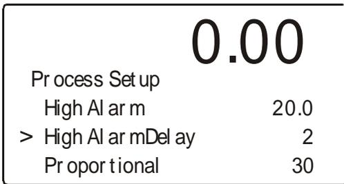
**FIG. 4-47 INSTRUMENT SETUP MENU/SETTING HIGH ALARM DELAY**
