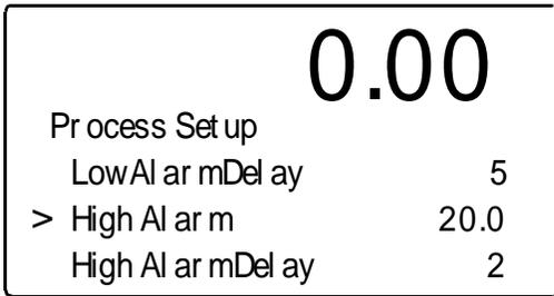
**FIG. 4-46 INSTRUMENT SETUP MENU/SETTING HIGH ALARM**
