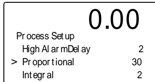
**FIG. 4-48 INSTRUMENT SETUP MENU/SETTING THE PROPORTIONAL VALUE**
