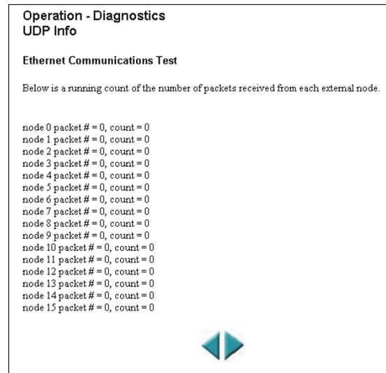
**FIG. 7-31 COUNT OF UDP PACKETS RECEIVED FROM EACH EXTERNAL NODE ON YOUR NETWORK**
