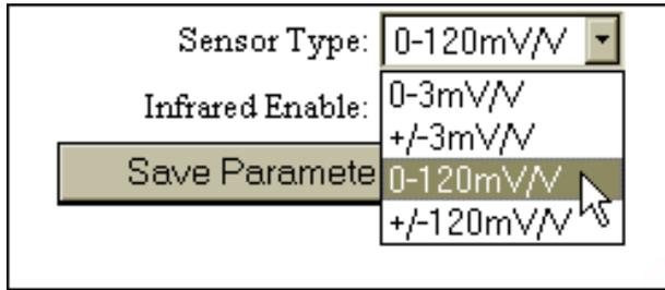
**FIG. 4-61 INSTRUMENT SETUP PAGE/SELECTING SENSOR TYPE**
