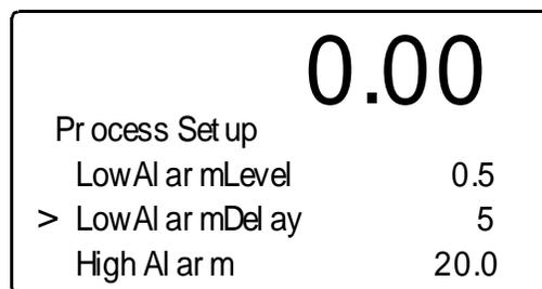
**FIG. 4-45 INSTRUMENT SETUP MENU/SETTING LOW ALARM DELAY**
