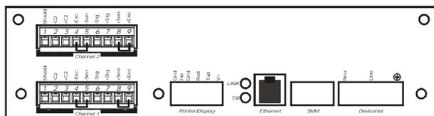
FIG. 3-19 LVDT CONNECTIONS/HI 3300 REAR PANEL
