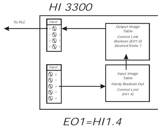
**FIG. 6-40 MAPPING CONTROL LOST INPUT TO CONTROL LINK BOOLEAN OUTPUT**
