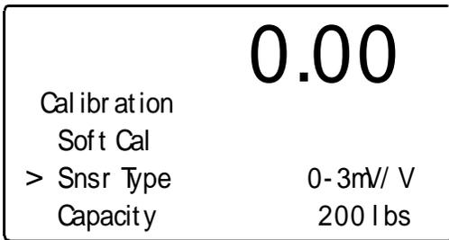
**FIG. 5-3 CALIBRATION/SELECTING SENSOR TYPE**
