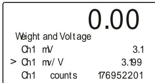
**FIG. 7-22 WEIGHT AND VOLTAGE MENU/CHANNEL 1 MV/V DISPLAY**
