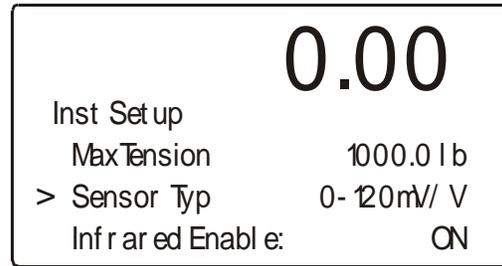
**FIG. 4-19 INSTRUMENT SETUP MENU/SENSOR TYPE**
