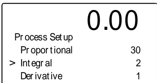
**FIG. 4-49 PROCESS SETUP MENU/SETTING THE INTEGRAL VALUE**
