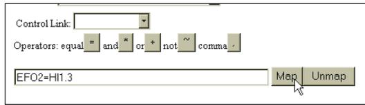
**FIG. 6-10 MAPPING HIGH TENSION ALARM TO CONTROL LINK FLOAT OUT**
