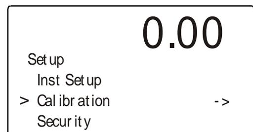
**FIG. 5-2 SETUP MENU/SELECTING CALIBRATION**
