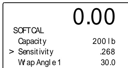
**FIG. 5-16 SOFT CALIBRATION MENU/ENTERING SENSITIVITY OF THE LOAD CELLS**
