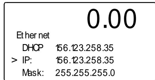
**FIG. 4-26 ETHERNET MENU/IP ADDRESS WITH DEFAULT IP ADDRESS**
