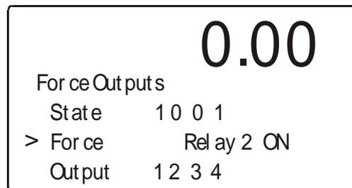
**FIG. 7-11 FORCE OUTPUTS MENU/SELECTING OUTPUT RELAY #2/ON**
