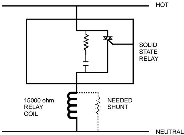
**FIG. 7-43 SCR SWITCHING LOAD CIRCUIT**
