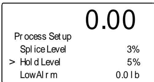
**FIG. 4-43 INSTRUMENT SETUP MENU/SETTING THE HOLD LEVEL**
