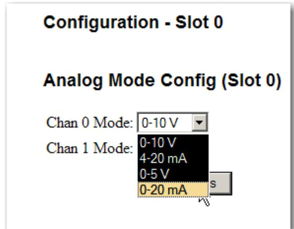
**FIG. 4-75 CONFIGURATION/SLOT 0/SETTING CHAN 0 MODE**
