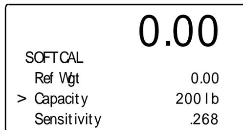
**FIG. 5-15 SOFT CALIBRATION MENU/ENTERING LOAD SENSOR CAPACITY**
