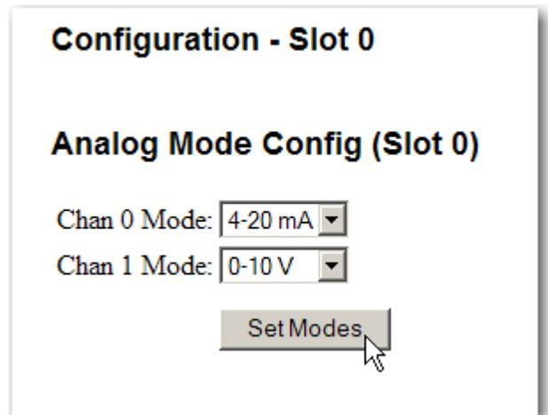
**FIG. 4-76 CONFIGURATION SLOT 0/SETTING MODES**
