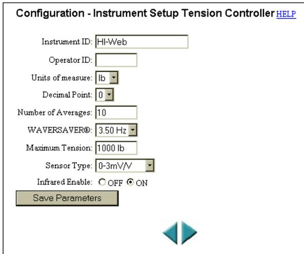
**FIG. 4-57 CONFIGURATION - INSTRUMENT SETUP TENSION CONTROLLER PAGE**
