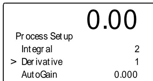
**FIG. 4-50 PROCESS SETUP MENU/SETTING THE DERIVATIVE VALUE**
