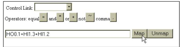
**FIG. 6-26 LOW TENSION ALARM (HI1.2) ADDED AS THE SECOND SOURCE TO THE ASSIGNMENT STATEMENT**
