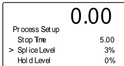
**FIG. 4-42 INSTRUMENT SETUP MENU/SETTING SPICE LEVEL**
