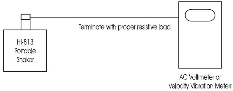
**FIG. 1-3 CHECKING VELOCITY TRANSDUCERS THAT ARE SELF POWERED**
