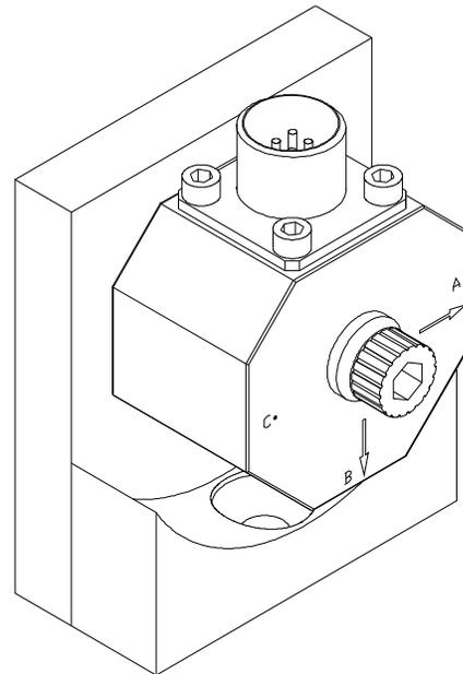
**FIG. 3-6 DI-103A B-AXIS POSITION WITH B ARROW POINTING DOWN**
